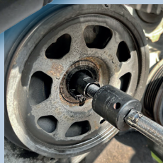
AST6245 VIBRATION DAMPER / CRANKSHAFT PULLEY REMOVAL TOOL - FORD 2.0 ECOBLUE RANGER & TRANSIT / HYBRID MHEV
