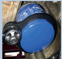
AST6176 OIL FILTER WRENCH - 74MM X 14 FLATS - 1.0 / 1.5 FORD - 1.0 / 1.4 / 2.0 OPEL/VAUXHALL
