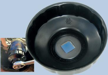
AST6089 OIL FILTER WRENCH - 76mm X 12 FLUTE - 1.0 FIREFLY PETROL ENGINE, 1.2GDI EB2 PETROL AND 1.5DCI K9K DIESEL -PSA - FIAT - FORD - JEEP - RENAULT - DACIA - MERCEDES-BENZ - NISSAN - VAUXHALL/OPEL 1/2" square drive - can be used with a standard 1/2" ratchet or extension bar.
